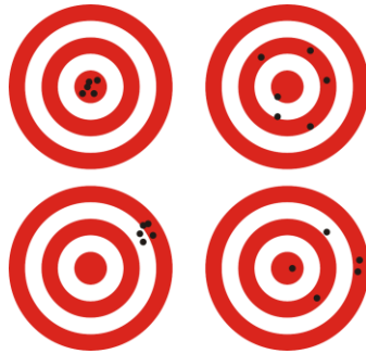
Figure 1. Accurate and inaccurate groupings of a precision firearm on the left, with accurate and inaccurate groupings of a less precise firearm on the right.
